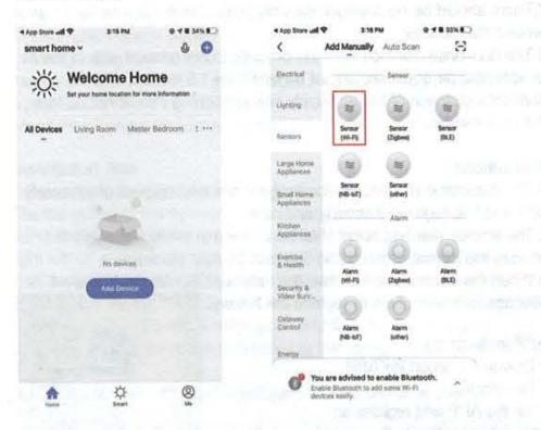
Install the battery to make the power on, press the button on the middle of the device and hold on for 5 seconds to enter into the Wi-Fi configuration state (the red standby indicator flashes fast indicates that it is in the smart link configuration mode. If the indicator light flashes slowly, it indicates it is in the AP configuration mode). There are two modes displays in the APP interface which can be switched to each other before configuration start. As below:
